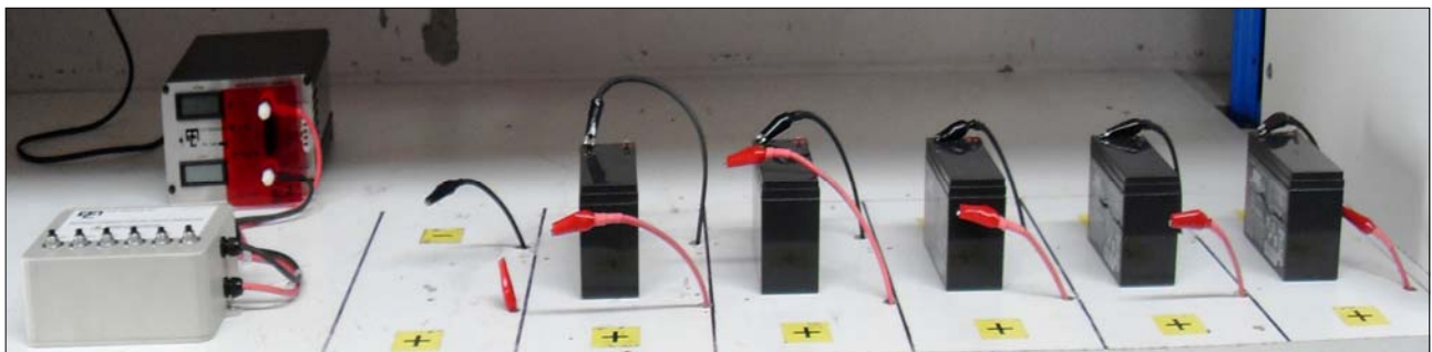
Figure 12: Charger Station & 5 Identical Batteries (Front View)
