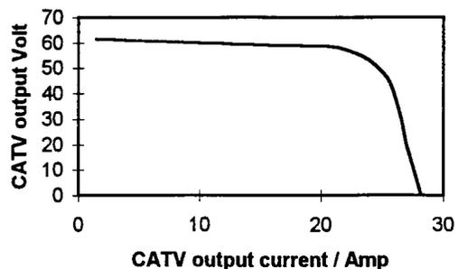
**Fig 4.** Foldback characteristics of a typical 15 amp FPS
