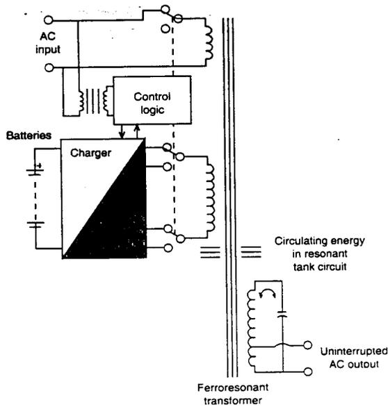
**Fig 10.** Single ferroresonant UPS functional block diagram
