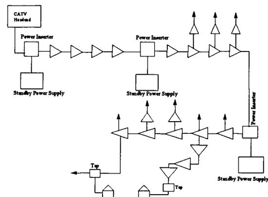
**Fig 1:** Tree and branch coaxial architecture
