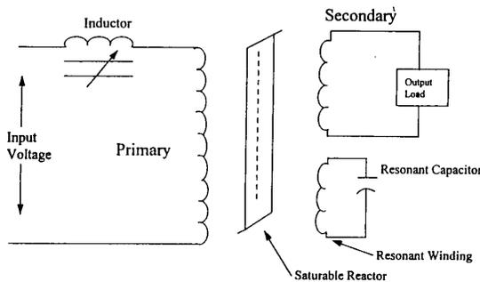
**Fig 2:** Simplified equivalent circuit of a ferroresonant transformer
