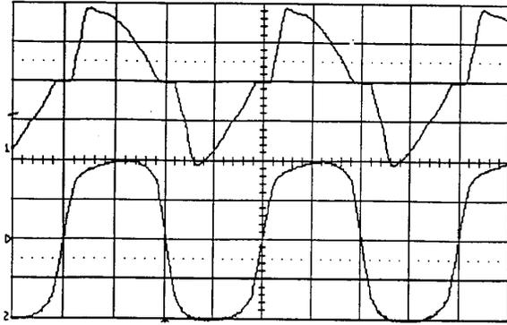
**Fig 8.** Current and voltage waveform for a 16.4 A load. (Scale: Current 20 A/div, Voltage 50 V/div)
