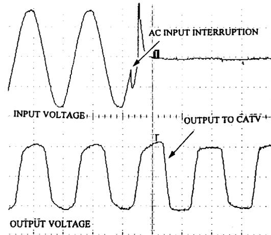
**Fig 9.** Standby FPS - Transfer from utility supply to battery
