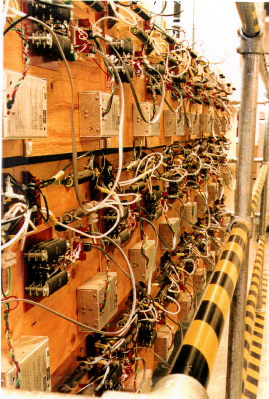
**Photo 1** The cascaded SMPS used for cable load simulation
