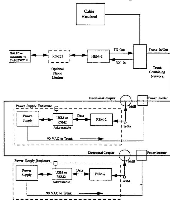
Fig 11. Status monitoring arrangement
