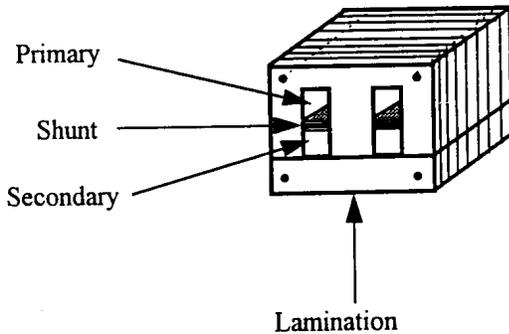
**Fig 3.** Construction of EI laminated ferroresonant transformer
